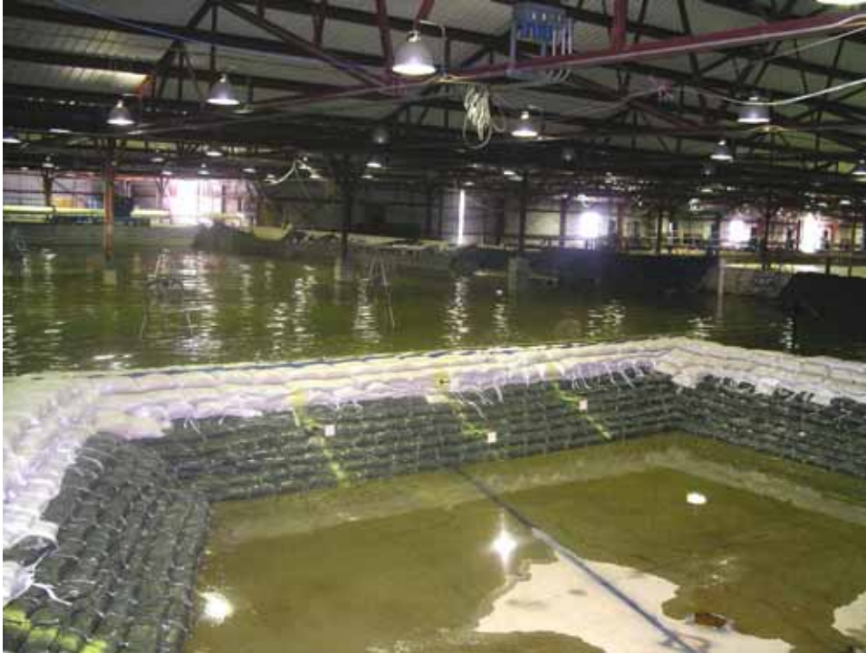
Figure 2-23. Sandbag levee with three of eight targets ready to test
