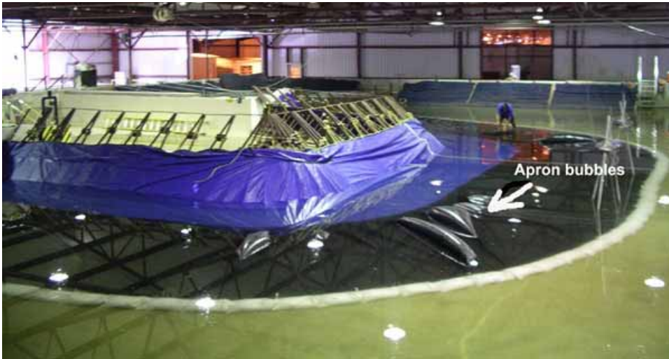
Figure 2-215. Air bubbles beneath apron
