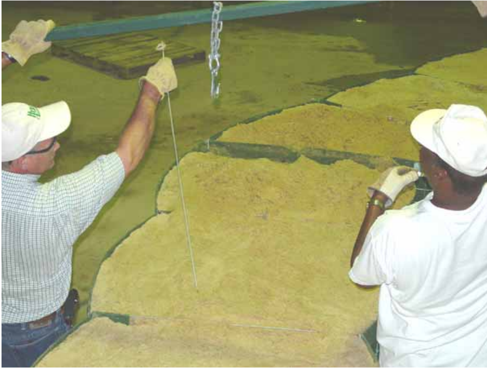
Figure 2-91. Removing center partition pin
