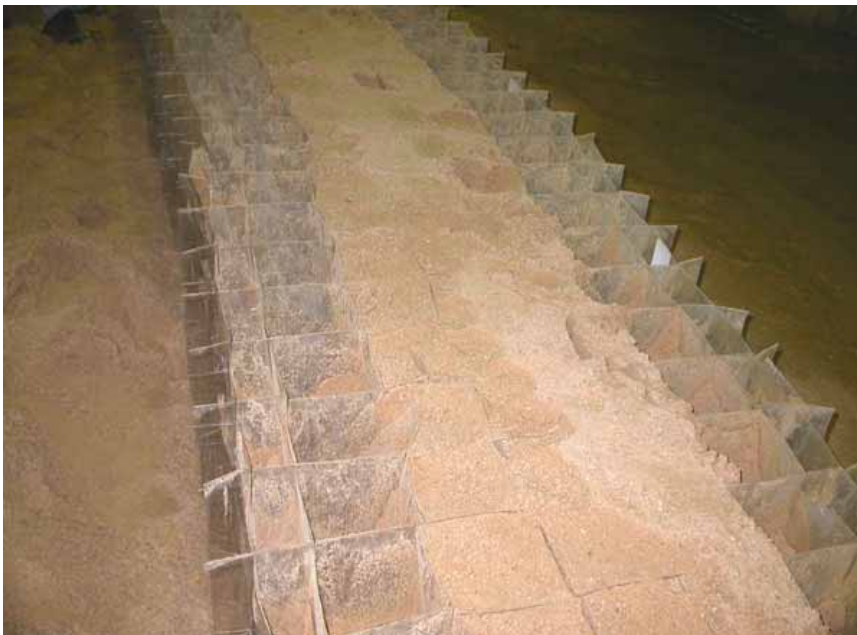
Figure 2-170. Removed sand from outer grid cells
