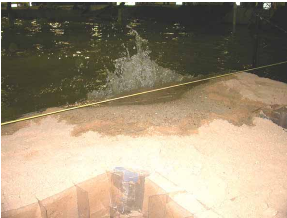
Figure 2-141. Wave impact against center wall
