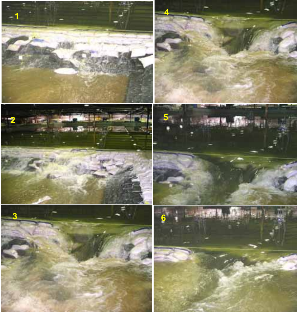
Figure 2-38. Sandbag levee progressive failure while testing
