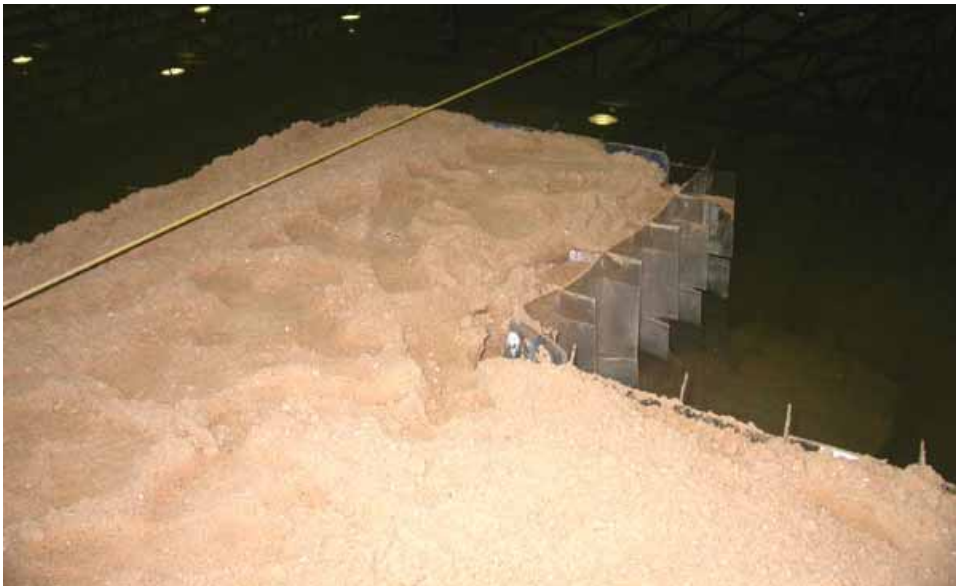
Figure 2-139. Right wall buttress
