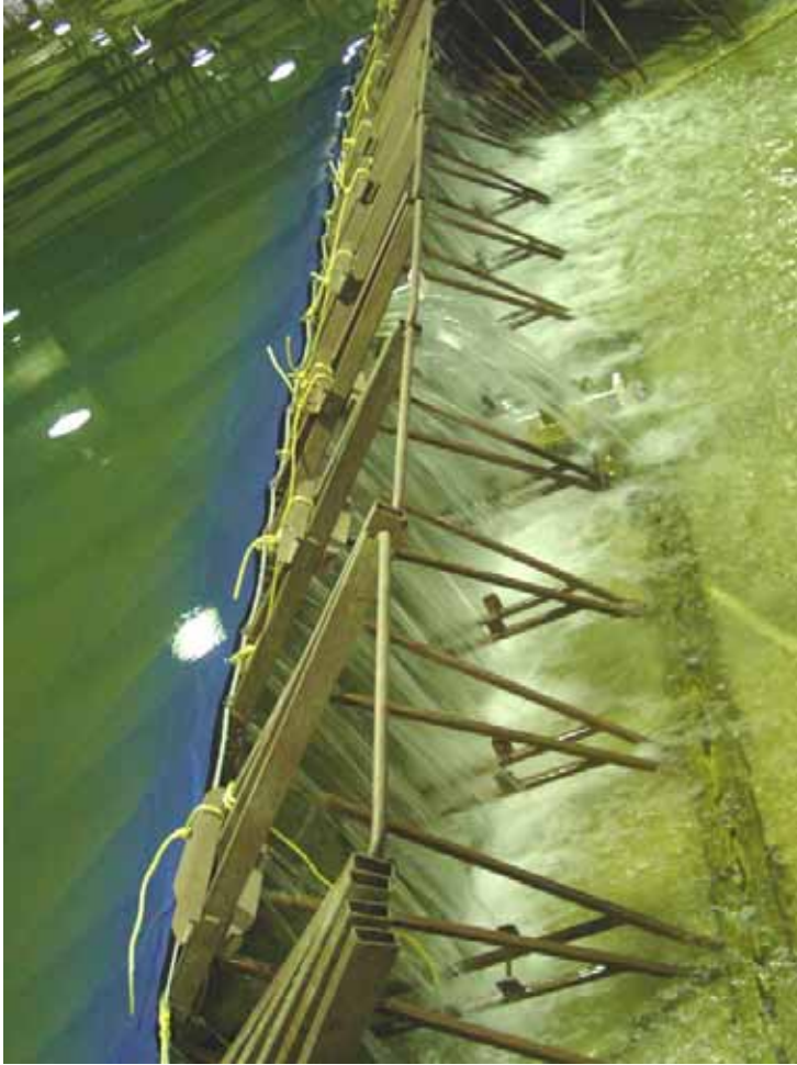
Figure 2-237. View of overtopped left wall
