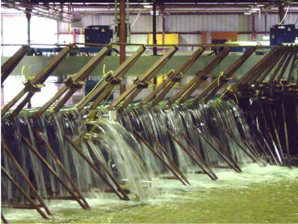
Figure 2-238. Center wall overtopping
