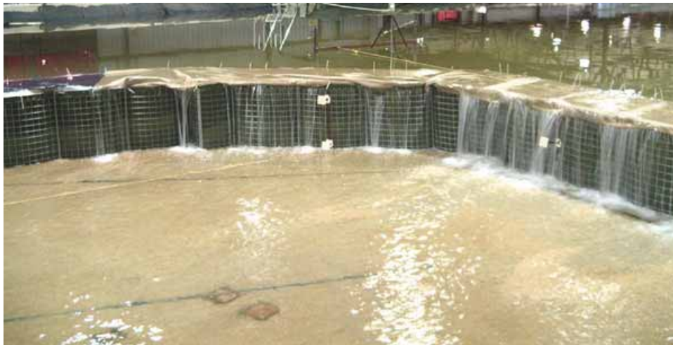
Figure 2-83. Overtopped levee structure, view from right wall
