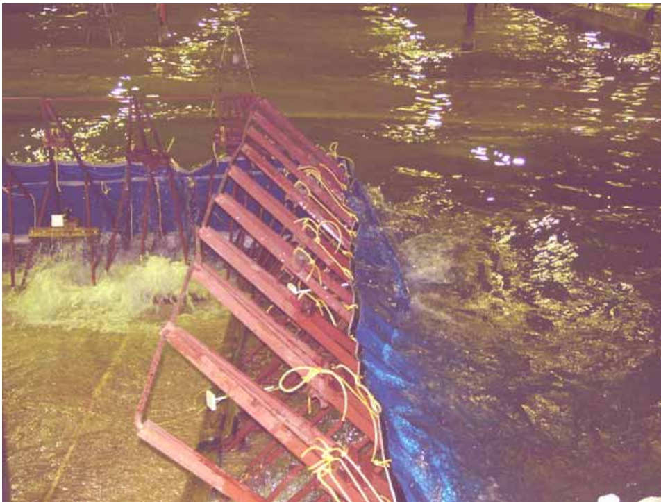
Figure 2-232. 7- to 9-in. wave test showing wave overtopping
