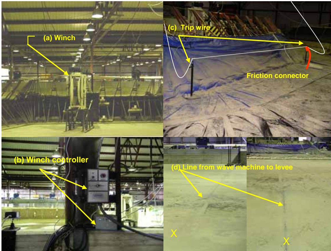
Figure 2-9. Debris impact test setup (a) Winch (b) Controller (c) Trip wire, (d) Desired path for log being towed
