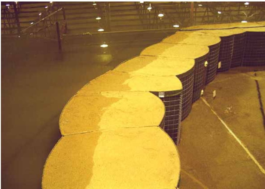
Figure 2-63. View of left wall water saturation
