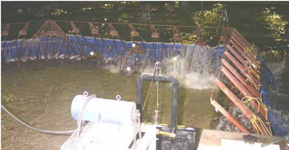
Figure 2-234. 10- to 13-in. wave test showing wave overtopping along center wall (partial view of impact test apparatus)
