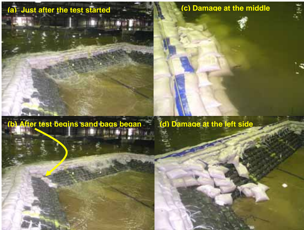
Figure 2-42. Damage to levee during the 10- to 13-in. waves, water at 80 percent of barrier height
