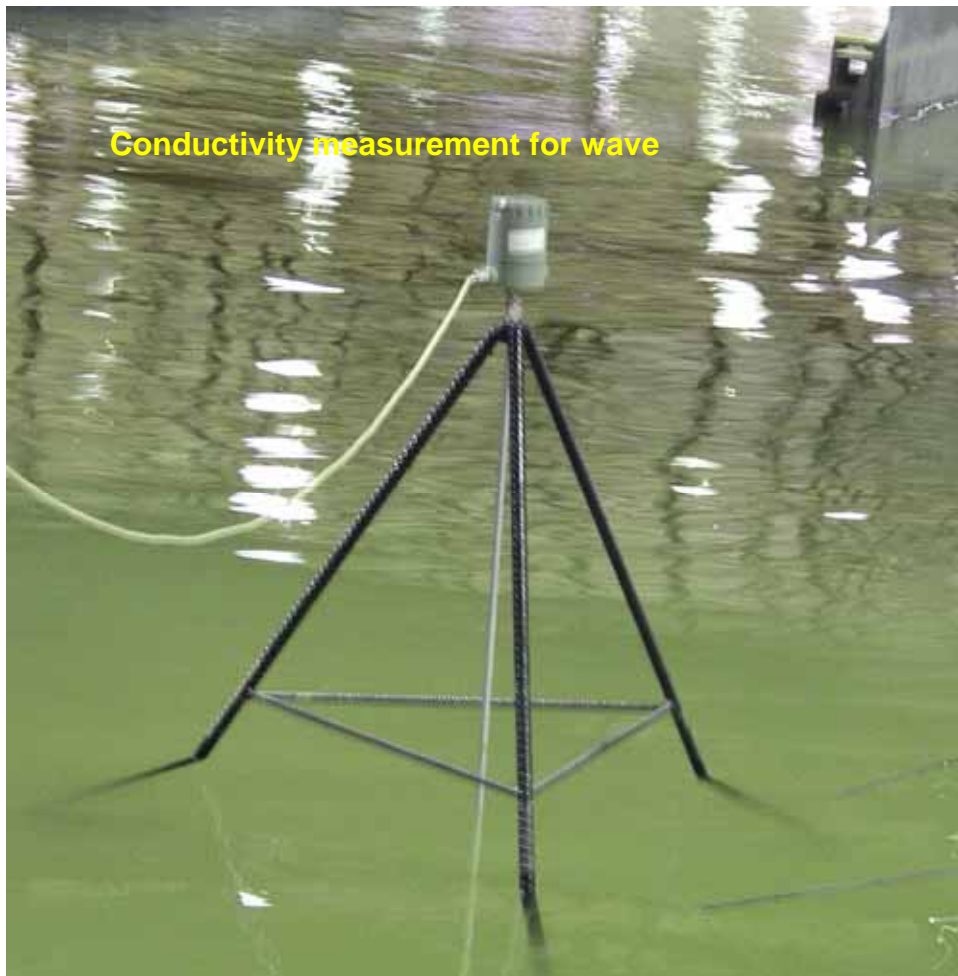
Figure 2-13. Separate wave conductivity rod, correlating waves with seepage
