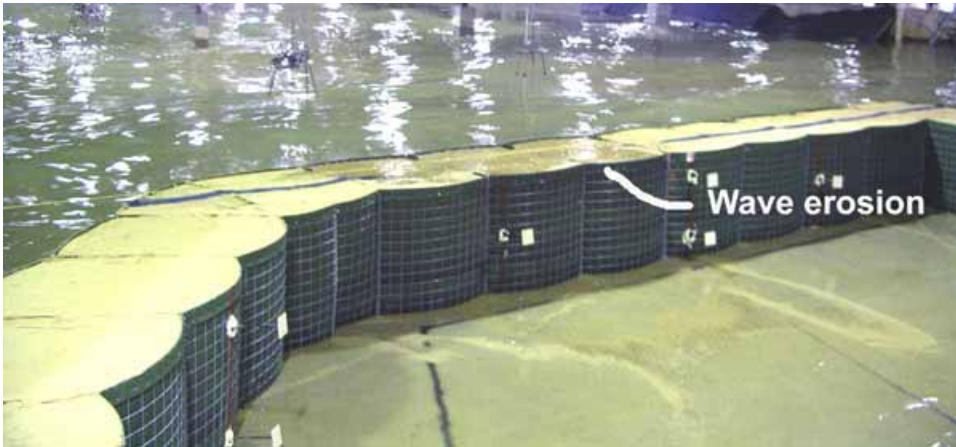
Figure 2-72. Center wall wave-induced erosion
