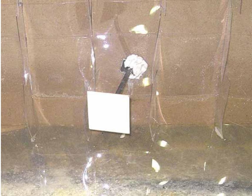
Figure 2-124. Typical laser target installation
