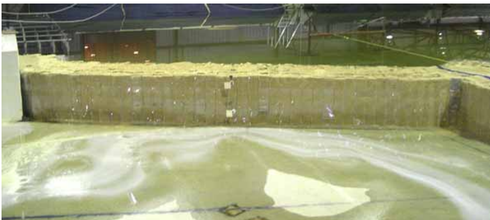
Figure 2-130. View of seepage under left wall
