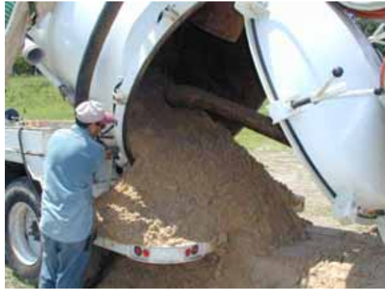
Figure 3-140. Removal of sand from truck
