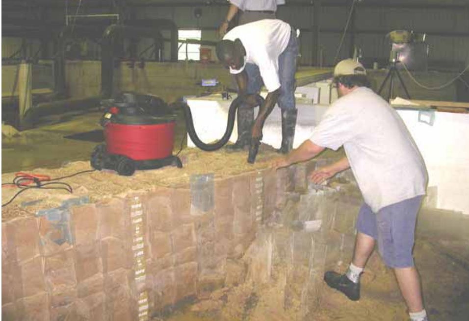
Figure 2-167. Removing sand from top of wall
