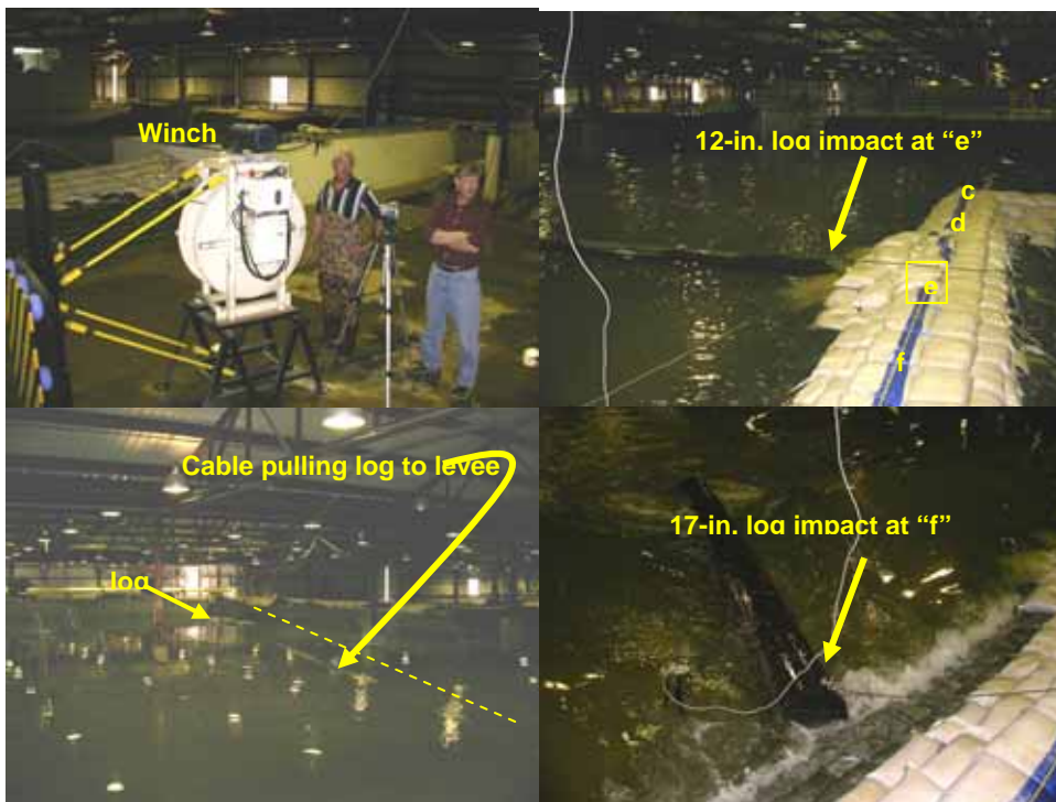
Figure 2-35. 12- and 16-in. logs at point of impact
