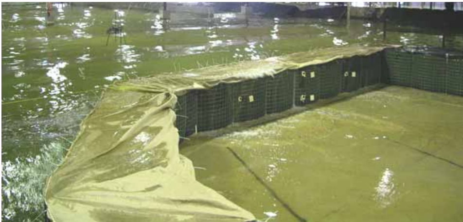
Figure 2-81. Wave overtopping along center wall
