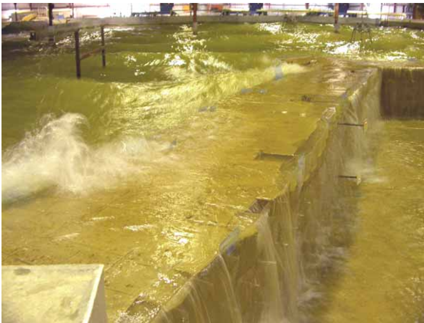
Figure 2-151. Waves overtopping left wall
