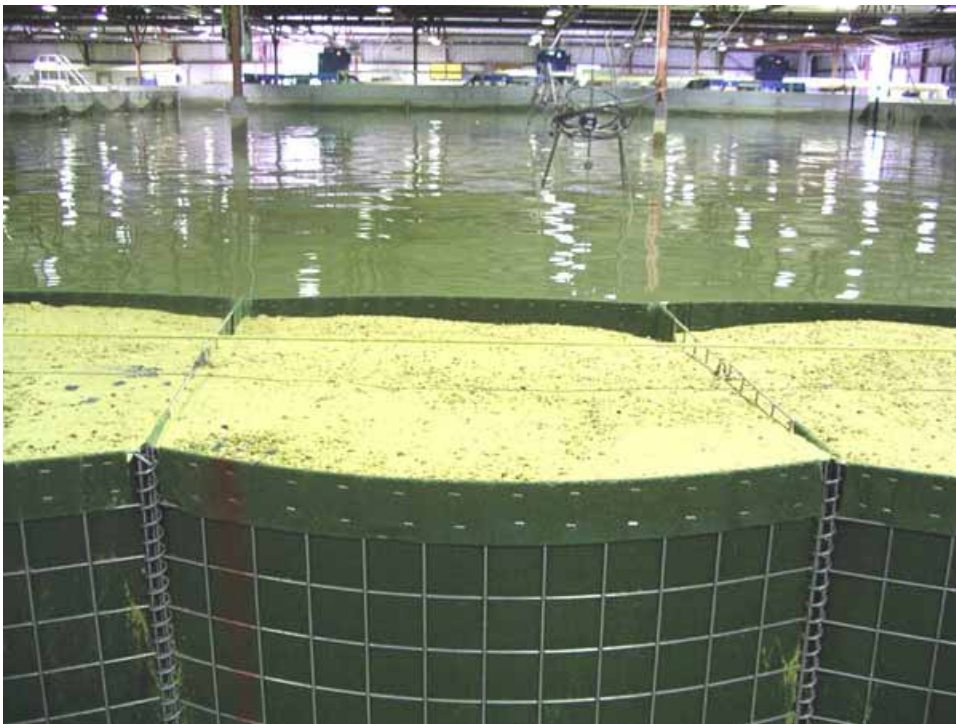
Figure 2-73. Sand eroded from top of center wall
