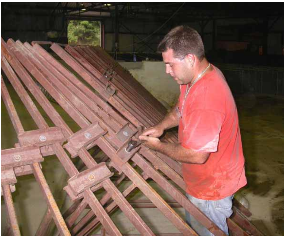
Figure 2-249. Disassembling frame brackets with socket wrench
