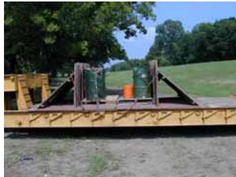
Figure 3-189. Loading Portadam frame members and hardware onto trailer
