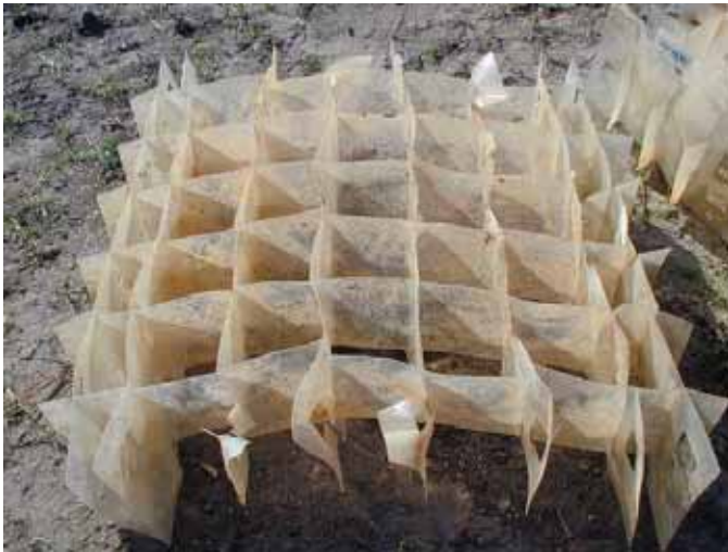
Figure 3-144. Damaged RDFW unit
