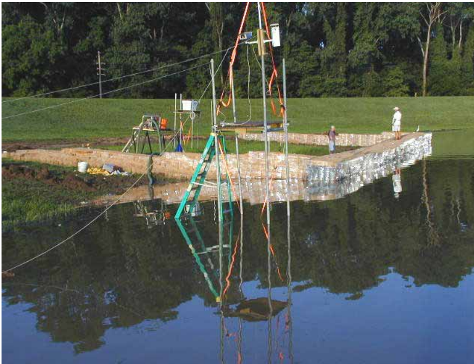
Figure 3-16. DAU mounted on an elevated stand
