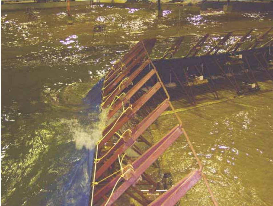
Figure 2-230. Aborted wave test showing wave overtopping along left wall
