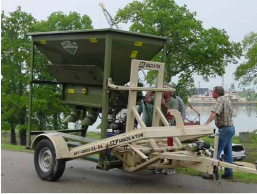
Figure 3-33. Hogan automatic-speed sandbagger as delivered to field test site
