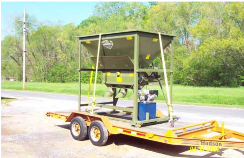
Figure 2-15. Hogan Manufacturing Co. sandbag filling machine used to build pretest sandbag levee
