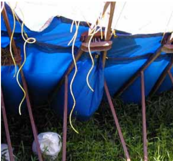
Figure 3-172. Sagging of liner between supporting frame members
