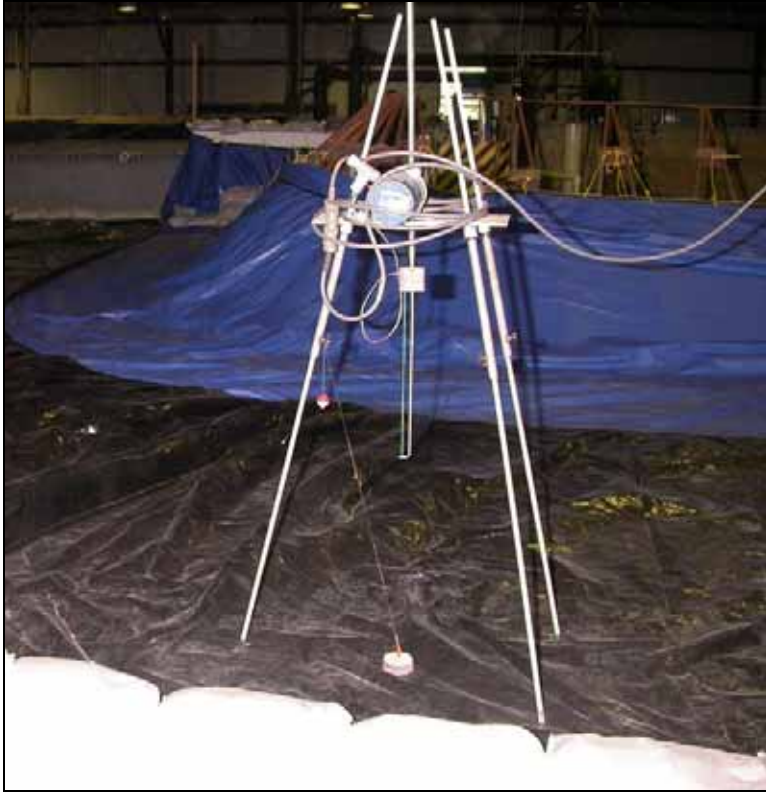
Figure 2-214. Pool elevation sensor placed on center apron
