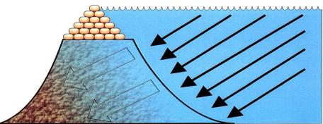
Infiltration of flood waters leads to saturation of the soils which can cause levee failure
