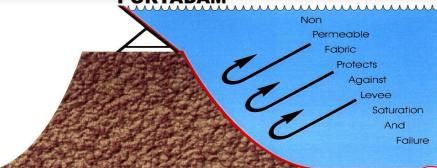
Portadam with extended liner not only raises the levee height, but helps to maintain levee soil stability
